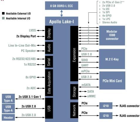
\*\*One PCIe x1 lane is software switchable to 1x USB 3.1 Gen 1
