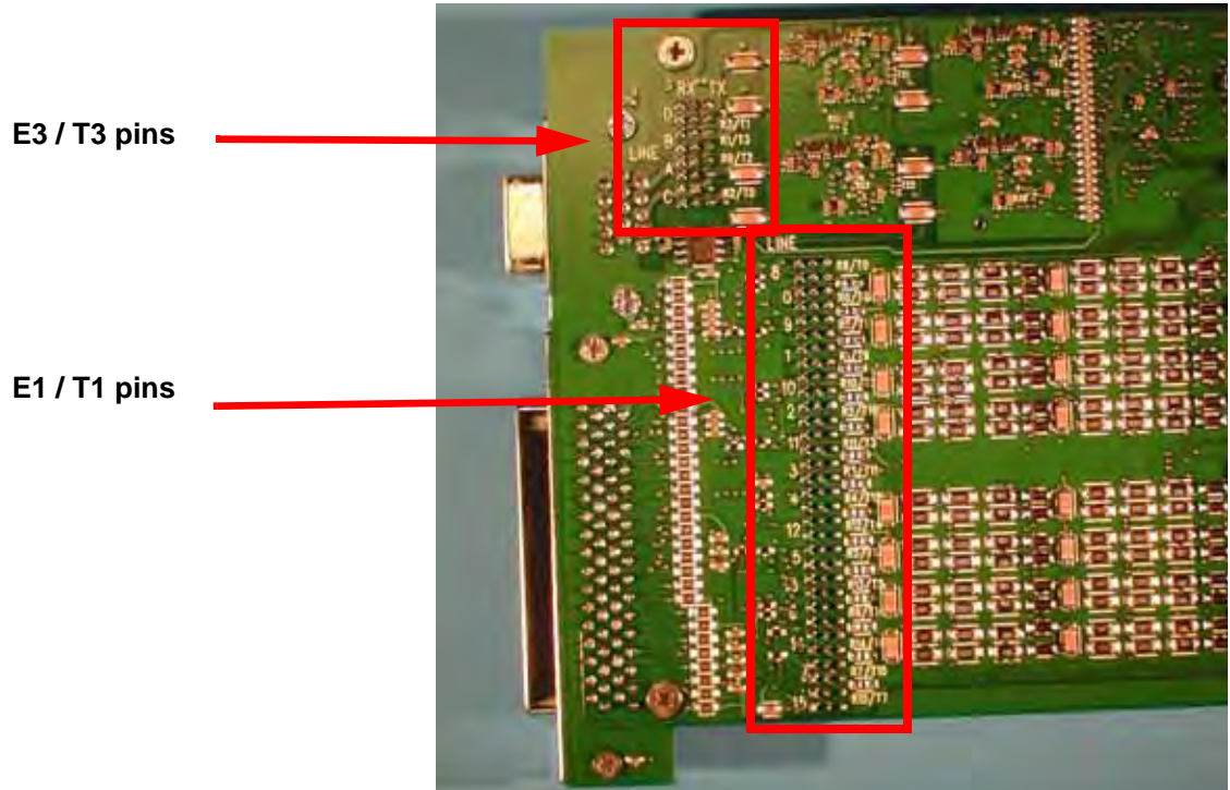
Figure 1. Combo and Combo 2 – Pin Locations and Legends
