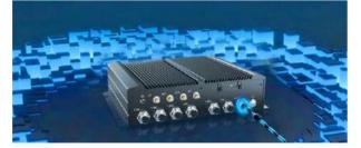
Adaptable Power Connectivity To address voltage fluctuations and different vehicle power specifications, our in-vehicle pcs incorporate a wide-voltage power input (8 to 36 VDC) and feature ignition control for ensuring power supply stability.
