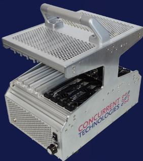
Vulcan is a ready-to-use solution for customers starting 3U VPX™ projects based on Intel® processor Plug In Cards.
